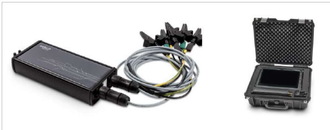
Figure 4.12. Portable XPM with computer for field measurements (data from Wideco Sweden AB)
