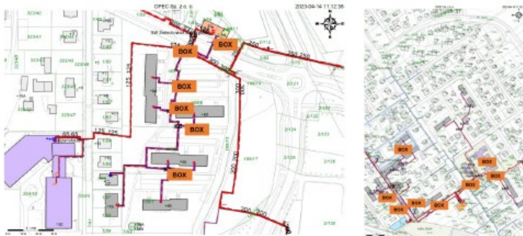
Figure 5.5. Locations of sensor stations (boxes) in Wejherowo, OPEC DH grid (photo by Gdańsk University of Technology)
