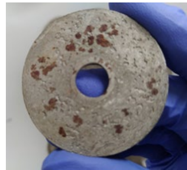
The indicator was removed from the pipeline after three years of use
