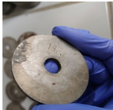
The indicator was removed from the pipeline after three years of use
